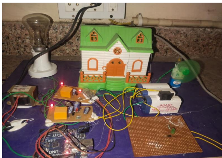
Fig 4.1 hardware model of solar home automation
